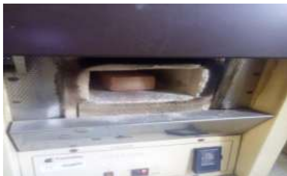
Fig. 3: showing brick in the muffle furnace.
